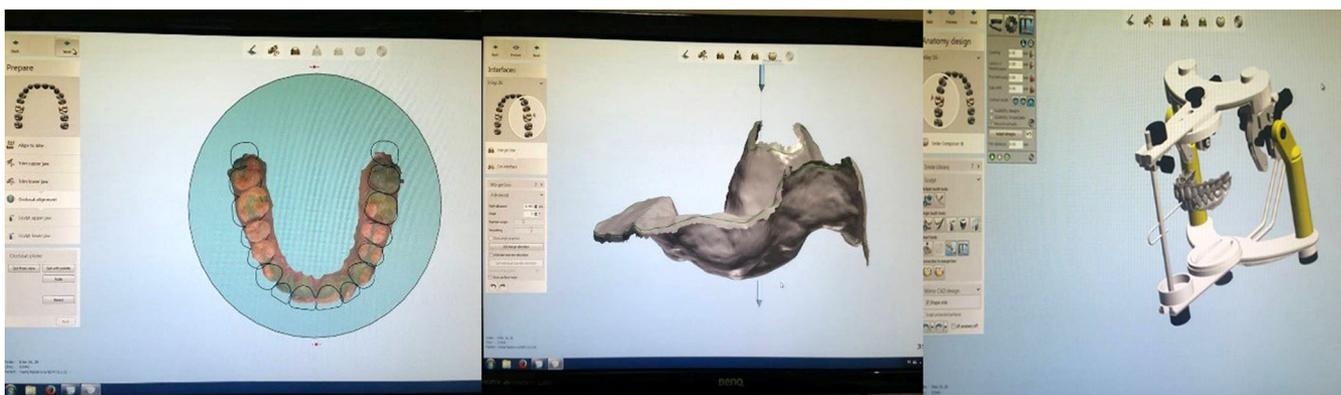
The designed restoration is situated on the disc and processed for milling by the CAM module (vhf milling machine). All restorations are made from Ultra Translucent Multi Layered (UTML) Zirconia discs (Kuraray Noritake Dental Inc.).
