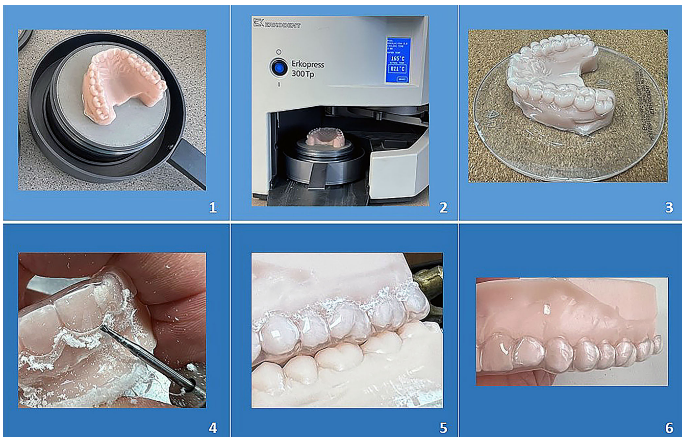
Fig. 4. Laboratory stages of manufacturing the mouthguard: 1) positioning of the model. 2) a thermopress machine. 3) molded plate. 4) cutting and shaping along the borders. 5) printing the antagonists. 6) the finished mouthguard.
