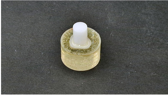
Fig. 1. The test specimens, composed of a dentin base to which a ceramic cylinder is bonded using a cement
