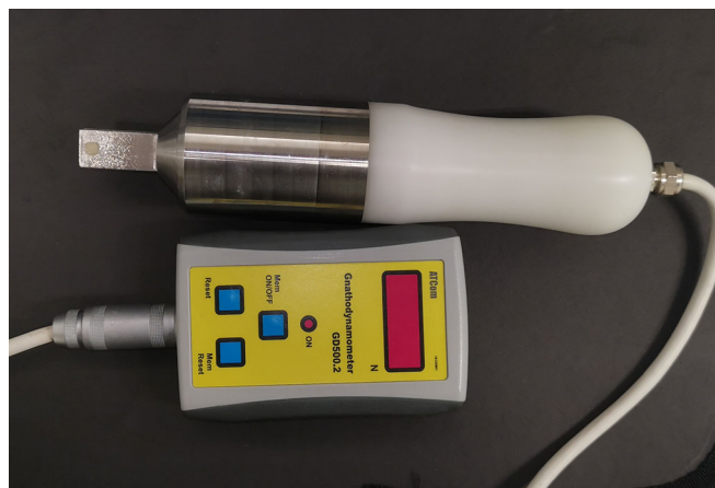
Fig. 2. Maximum bite force testing.
