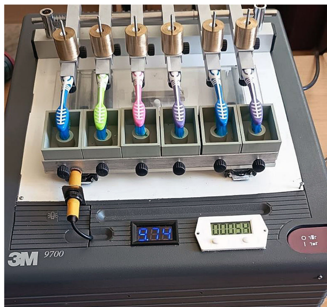
Fig. 1. Custom-designed machine for simulated toothbrushing.
